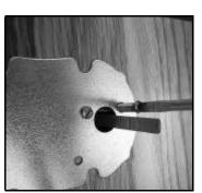
Position the steel back-plate on the inside of the door. Insert the 2 connecting screws into the holes adjacent to the large hole in the center of the back-plate and thread them into the holes in the back of the cylinder. Using a screwdriver, tighten the screws, making sure the back-plate is positioned 1/8" from the edge of the door and the 4 small mounting holes are accessible.
