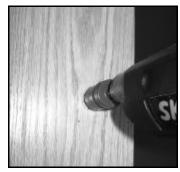
Drill the 1-3/8" diameter hole through the door. Take care to ensure that the drill is mevel and the hole is straight through the door. (TIP: Bore the hole to the point of the tip, breaking through the opposite side and finish boring out the hole from the opposite side to reduce splintering the door.)
