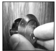
Slip the cylinder collar over the cylinder and insert the cylinder into the door from the exterior. Position the keyhole at the bottom of the lock with the SEGAL\* trademark at the top. Hold cylinder in place.
