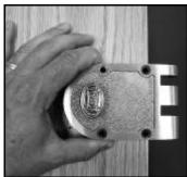
With the deadbolt in the unlocked position, push and hold in the shutter guard and place the lock case over the back-plate (on the inside of the door.) Make sure the tailpiece goes into the hole on the back of the lock (as exposed by the shutter guard.)
